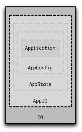
Figure 7.9: Graphical representation of the App monad stack within which framework applications execute. The AppIO monad encapsulates applications, preventing them from calling unsafe functions within the IO monad.
