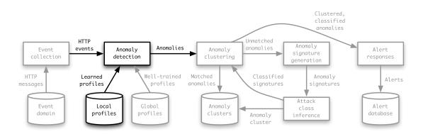
Figure 6.5: Architectural overview of WEBANOMALY, with concept drift components highlighted.
