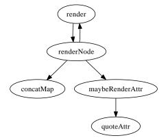
Figure 7.12: Example control flow graph for Render Node instance.
